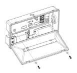
2 - Using one of the various fixing points, install the luminaire in its desired position, with the supply cables coming into the luminaire.
