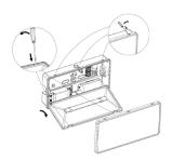
1- Using a terminal driver, open the cover, uncliping at all six points and remove it. With the same driver, upclip the geartray and swing it open at the hinge.
