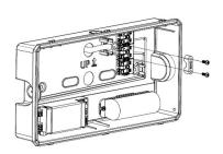
3 - Connect the supplies and, where required DALI bus. Once power is assured, connect the battery connector. Ensure that the cable clamp is tightened.
