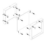
4 - Slide the legend panel into the frame fitting base (1) first and then top (2), connect earth lead from frame to base and fit frame to base. Tighten the side screws (3) to secure the frame and legend to the base
