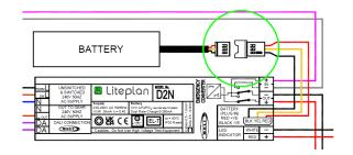
3 - Once permanent power is assured, connect the two three-pole battery connectors together.
