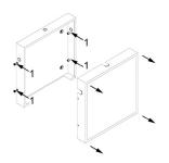
1- Take the fitting apart by loosening 4 screws (1) and pull frame and legend panel away. Unplug earth lead. Fix base to the wall using the four fixing points. Bringing in supply cable through the various entries.
