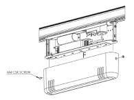
6 - If using the M4 screws, fit the cover, ensuring that the charge indicator is visible through its locator and fit the M4 counter sunk screws to hold the cover in place.
