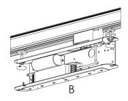
2 - Tighten the twist brackets in place using a pozidrive screwdriver. Enter the commissioning date to the label on the battery and connect the 3-way battery connector.
