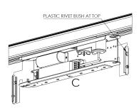
3 - If using the flush fixings, the side brackets should be fitted with the plastic bush at the top.
