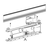
1- Fit the track adaptor in place, set the required circuit and offer the body of the EMTrac to the track.
