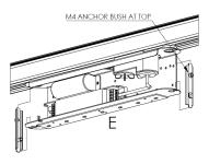
5 - If using the counter sunk screws, the side brackets should be fitted with the M4 anchor bush at the top. Figure six
