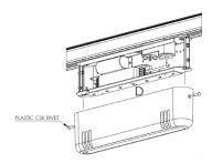
4 - If using the flush fixings, fit the cover, ensuring that the charge indicator is visible through its locator and push the plastic counter sunk rivets into place to hold the cover.
