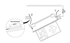
6 - Install the assembled CE1R into the ceiling cutout. A minimum void depth of 125mm must be observed.
