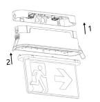
5 - Click the body back into the first fix section, ensuring the the connector(s) from the mains/DALI terminal blocks have been connected to the gear tray. Click the legend to the body ensuring it is the correct way round and oberving the position of the charge LED. Figure six
