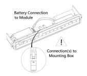
3 - Once mains supply is present, connect the 3-way battery cable connector together.
