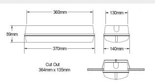
The OLP/1 is a high quality emergency LED bulkhead which is designed for interior and exterior applications.
