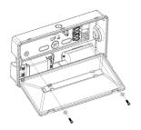
2 - Using one of the various fixing points, install the luminaire in its desired position, with the supply cables coming into the luminaire.
