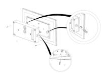
1- Take the fitting apart as shown in the above diagrams, removing the back box from the main body of the exit sign.
