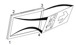
6 - Fit the legend vinyls to the body of the CE2S, starting at corner 1, then corner 2, then 3, then 4, observing the requirements of BS (EN) 5266.
