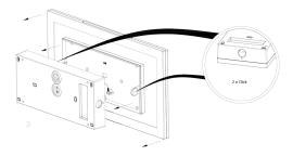
5 - Click the main body of the CE2S to the back box listening out for two clicks. Where required, add two security screws at the dimples.
