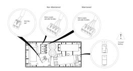
3 - Fit mains supply cables to the terminals as shown. Either maintained or non-maintianed as indicated and fit DALI cables if required. (DALI versions only).
