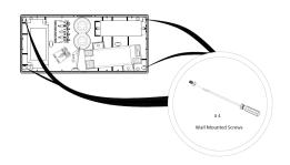
2 - Install the first fix section of the CE2S to wall, using either fixing points A or B.
