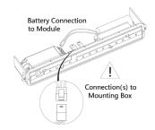
3 - Once mains supply is present, connect the 3-way battery cable connector together.
