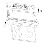
5 - Click the body back into the first fix section, ensuring the the connector(s) from the mains/DALI terminal blocks have been connected to the gear tray. Click the legend to the body ensuring it is the correct way round and oberving the position of the charge LED.
