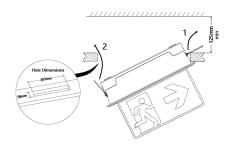
6 - Install the assembled CE1R into the ceiling cutout. A minimum void depth of 125mm must be observed.
