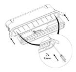
4 - Fit the gear tray back into the body, tightening the screws as shown.
