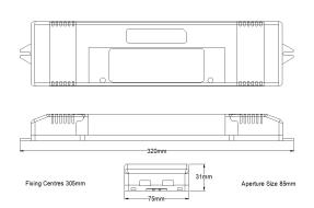
The TLP/2/SP85/R is supplied as a remote conversion kit designed to be mounted adjacent to the luminaire, where room inside the fitting is limited. This unit offers a higher output which is more suitable for higher power luminaires.
