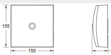
The Halo Surface Square is a square, surface mount standalone emergency LED luminaire which incorporates either our open area or corridor LEDs. The unit is designed for non-maintained use.
