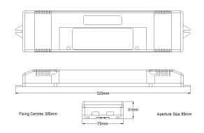
The D2N/2/SP85/R is supplied as a remote conversion kit designed to be mounted adjacent to the luminaire, where room inside the fitting is limited. This part offers a higher output which is more suitable for higher power luminaires.
