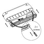
5 - Fit the gear tray back into the body, tightening the screws as shown.
