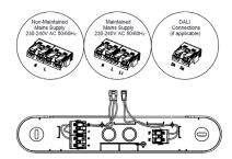
3 - Fit mains supply cables to the terminals as shown. Either maintained or non-maintianed apperation. Connect DALI cables if required. (DALI versions only).
