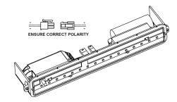
4 - Once mains supply is present, connect the battery cable connectors together.
