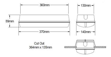
The OLP/1/MYMESH is a high quality emergency LED bulkhead which is designed for interior and exterior applications. The high output LED strip provides 1163 lumen in mains operation and 358 lumen in emergency operation after the diffuser.
