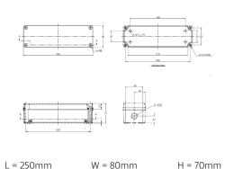
The D2N/2/WP100/R is supplied as a remote conversion kit for mounting away from the fitting in damp locations. This kit would be used in applications where space inside the fitting is limited.
