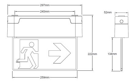
A stylish and compact Double Sided LED Exit Sign suitable for either wall or ceiling mounting. The unit is available in either a Switchable Maintained or Non-Maintained operation and is ready to connect to the MyMesh Wireless platform. The fitting is supplied with a PMMA screen printed legend plate which offers an impressive 25m viewing distance.
