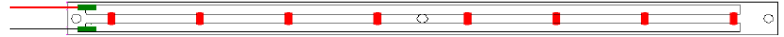
8 x Samsung 5630 - Pcb 304mm x 15mm - Fixings Centres 296mm - 250mm Red & Black Leads Constant Current 700mA - 1S8P - Max Rating 2.1 Watts - 6000K
