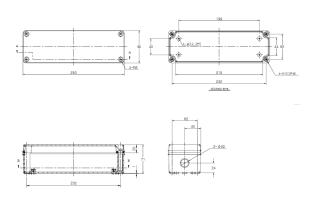
The NLP/2/WP100-R is supplied as a remote conversion kit designed to be mounted in wet or damp locations, adjacent to the luminaire, where room inside the fitting is limited. This part offers a higher output which is more suitable for higher power luminaires.
