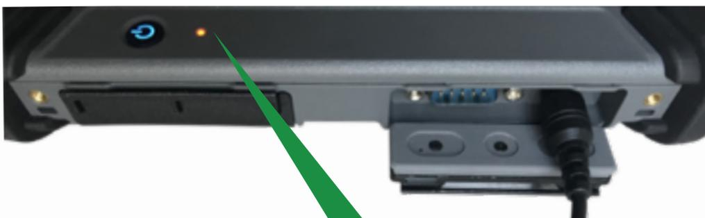
To charge, place the charging lead into the point as shown. When the tablet is charging, this light will be illuminated.
