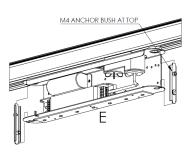
5 - If using the counter sunk screws, the side brackets should be fitted with the M4 anchor bush at the top.
