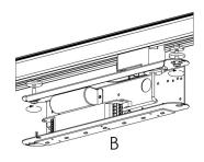
2 - Tighten the twist brackets in place using a pozidrive screwdriver. Enter the commissioning date to the label on the battery and connect the 2-way battery connector.
