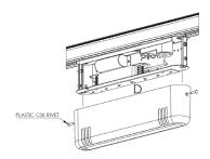
4 - If using the flush fixings, fit the cover, ensuring that the charge indicator is visible through its locator and push the plastic counter sunk rivets into place to hold the cover.
