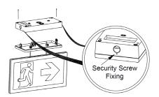
5 - Click the main body of the CE2S/SM to the back box listening out for two clicks. Where required, add two security screws at the dimples.
