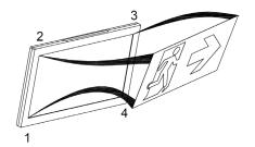
6 - Fit the legend vinyl to the body of the CE2S/SM. Start at corner 1, then corner 2, then 3, then 4, observing the requirements of BS (EN) 5266.
