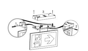
1- Take the fitting apart as shown in the diagrams above, removing the back box from the main body of the exit sign.
