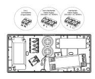
3 - Fit mains supply cables to the terminals as shown. Either maintained or non-maintianed as indicated and fit DALI cables if required. (DALI versions only).
