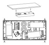
2 - Install the first fix section of the CE2S to the ceiling, using either fixing points A or B.
