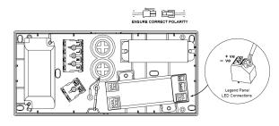
4 - Once mains supply is present, connect the battery cable connectors together and connect the LED leads from the panel to the module, as shown.
