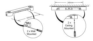
2 - Install the first fix section of the CE1S to either the wall, or the ceiling, as shown.
